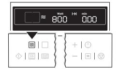
Using the + or - button, set the desired cooking time. The symbol for Cook time [+] flashes.
